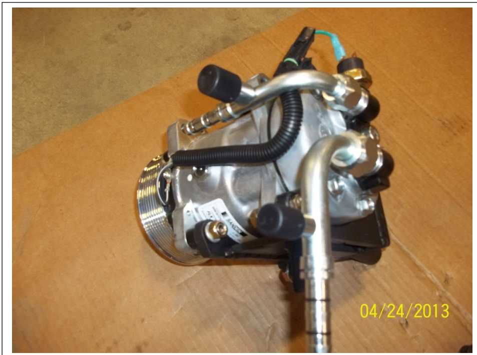
Most likely fitting set up at compressor.
