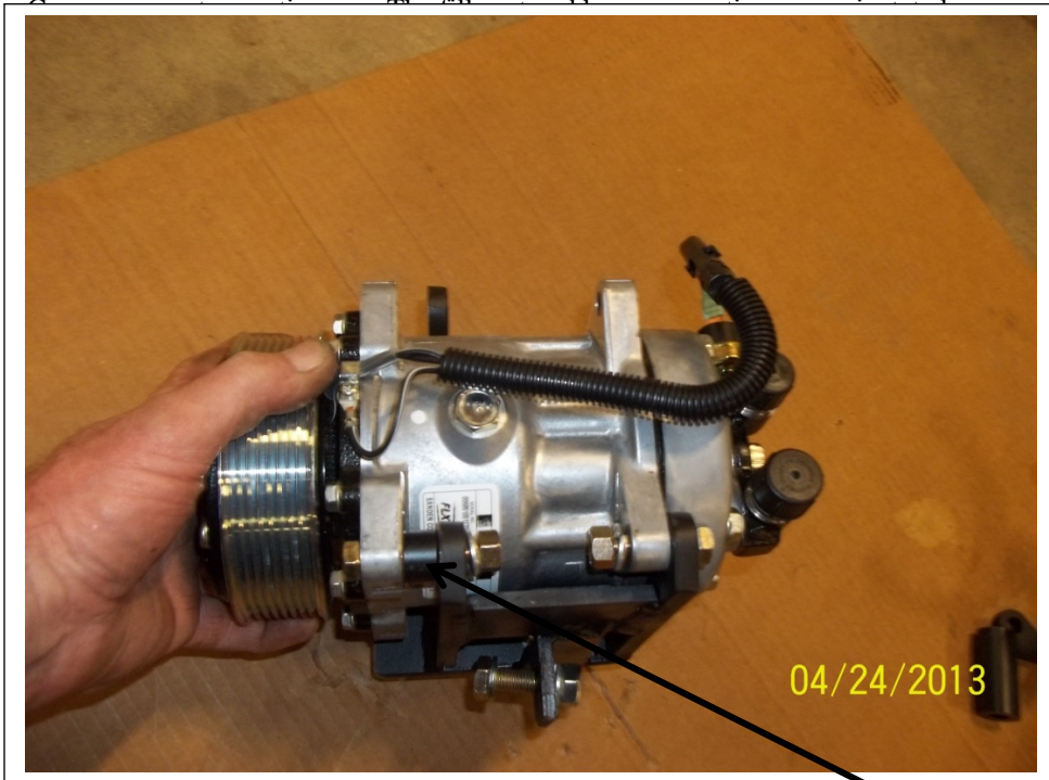
Most likely compressor set up. The oil plug and fittings are orientated away from the engine.
